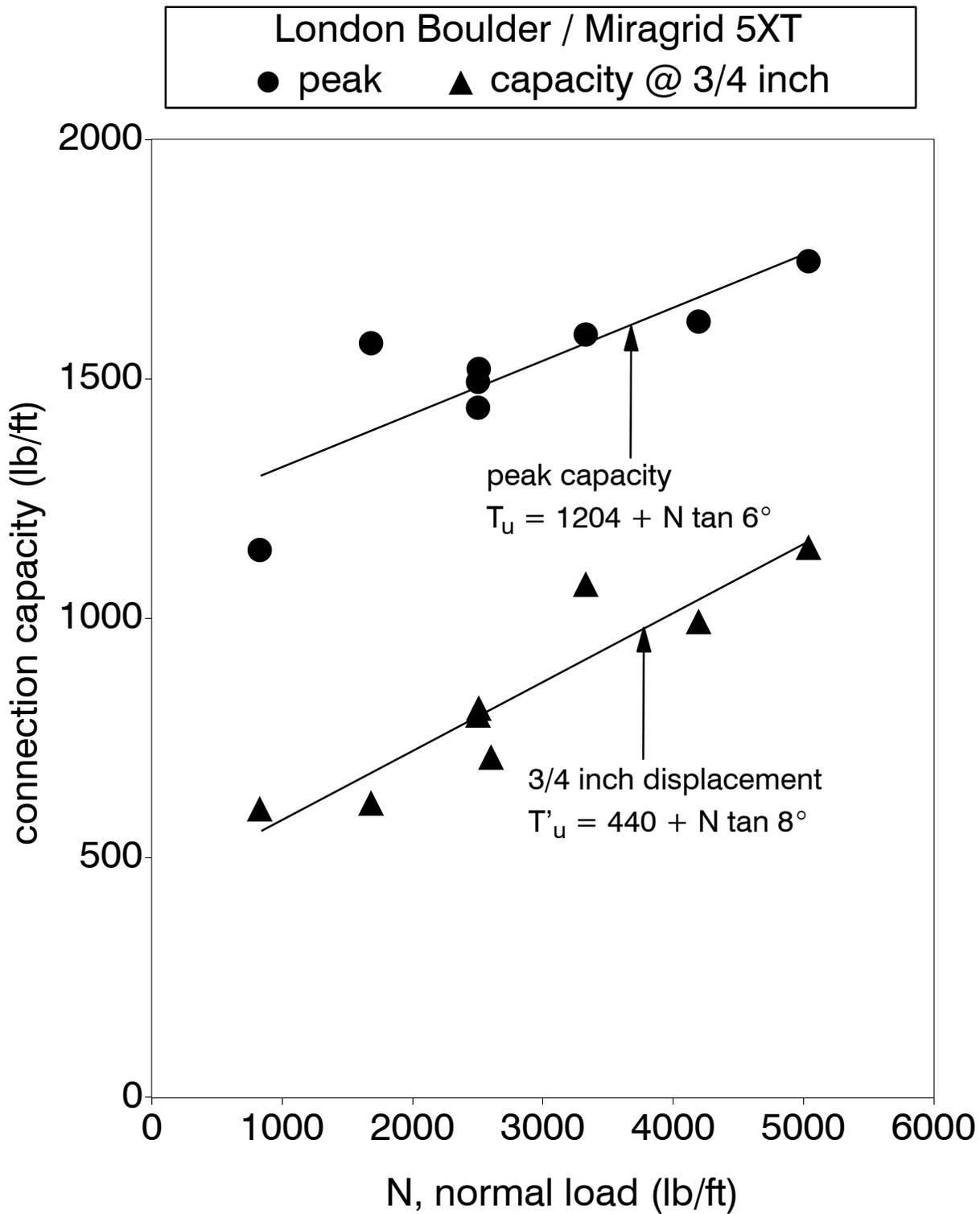
Figure 4: Summary of connection capacities for London Boulder block units (underside hollow section filled with concrete) and Miragrid 5XT geogrid
