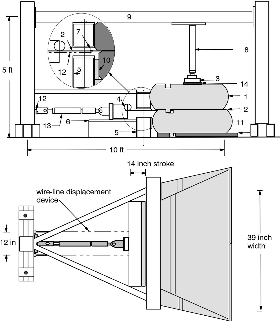
Figure 1: Schematic of connection test apparatus showing London Boulder units and Miragrid 5XT reinforcement
