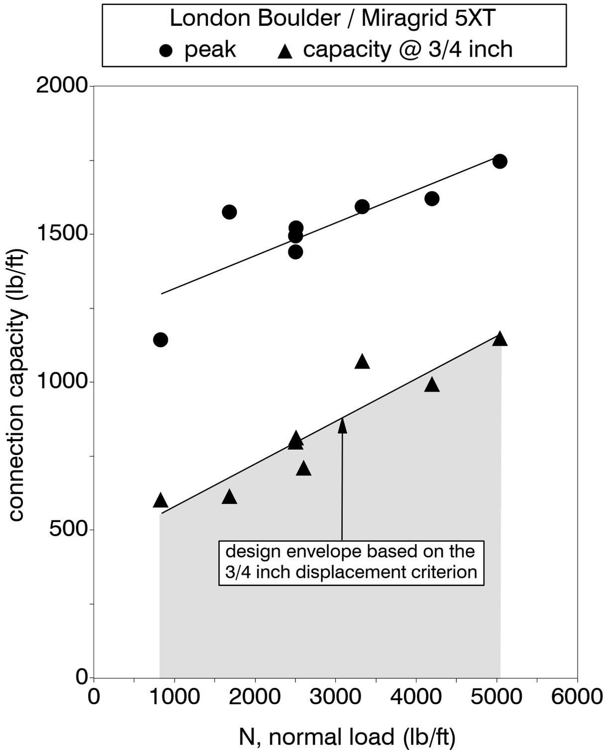
Figure 5: Design envelope for London Boulder blocks with Miragrid 5XT
