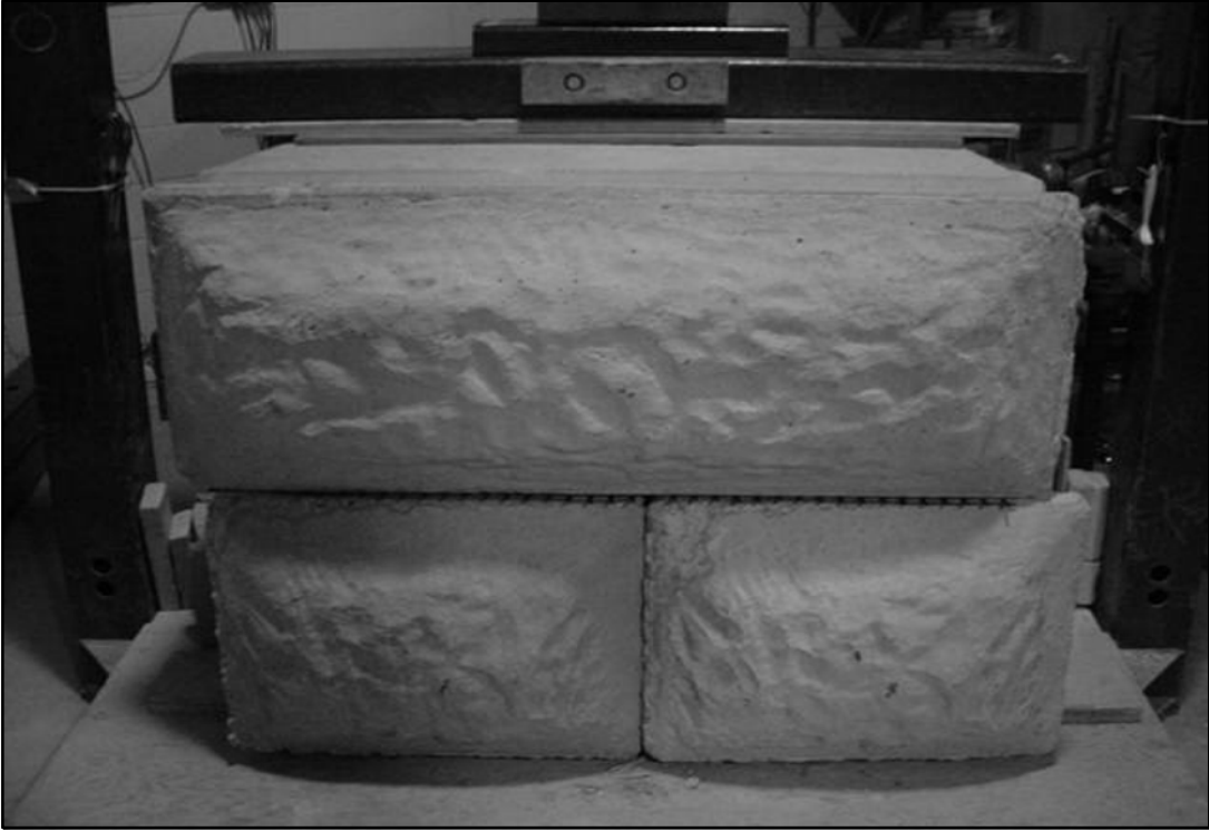
Figure 2: Photograph of the London Boulder block in the connection test apparatus
