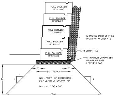
LONDONBOULDER - 2-INCH SETBACK I:I EXCAVATION OVERSIZING - GRAVITY WALL (NOT TO SCALE)
